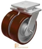
Double link wheel without brake, plate, wheel diameter 300 mm, building height 375 mm, hub in cast iron with soft track in PUR in red color. 3900 kg load capacity, double ball bearings
